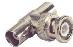
BNC tee—required on the back of the NIC
