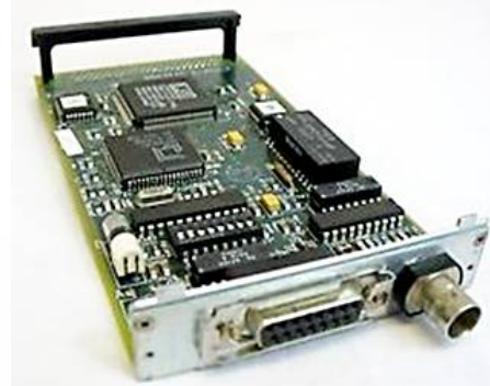
NIC with AUI (connects to a MAU) and thin Ethernet connectors.
